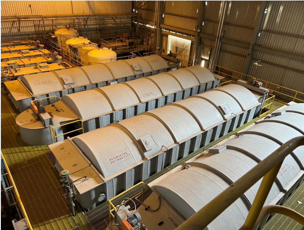
Figure 8: - Solvent extraction tanks/circuit show in very good condition – the end of this circuit is where the end-product is produced
