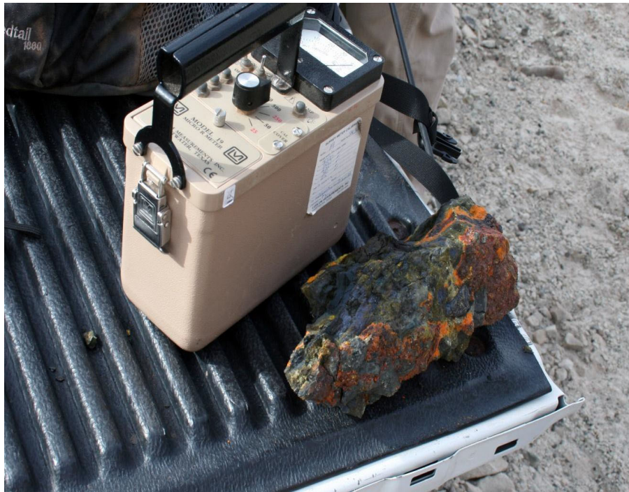
Figure 8.3 – Slick Rock Sample and Scintillometer
